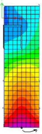
Plan View - OHT_LMR - Z = 23.2 (m) - Displacements (D+L) [mm] Story Response
